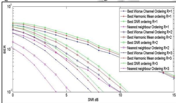
Figure 5. Comparison of four single RS schemes with relays=1,2,3
