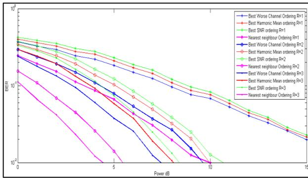
Fig. 4: Comparison of Four Single RS Schemes with Relays=1,2,3
