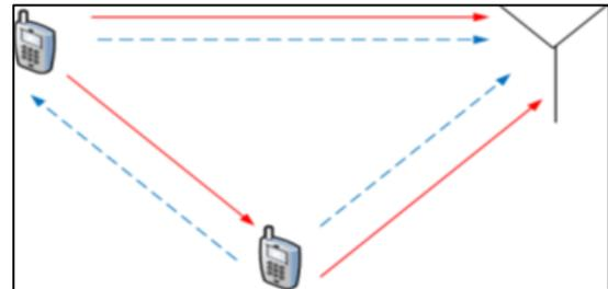
Fig. 2: In Cooperative Communication Each User is both a Source & a Relay
