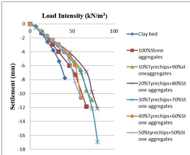
Fig. 2: Load settlement Graph of Single Column
