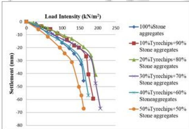
Fig. 3: Load settlement graph of two columns
