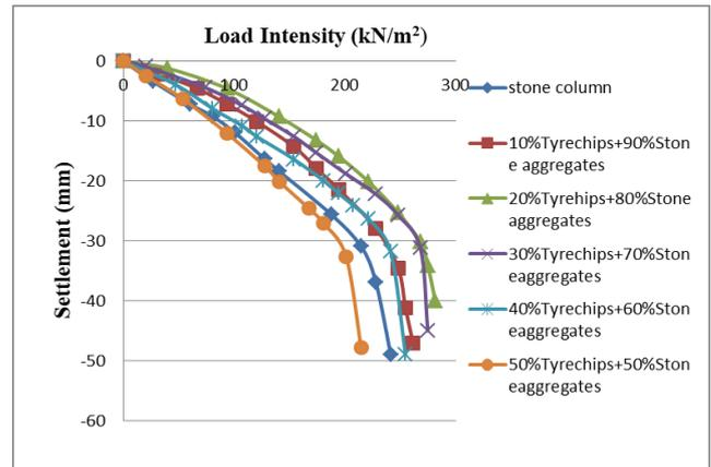
Fig. 4: Load Settlement Graph of Three Columns
