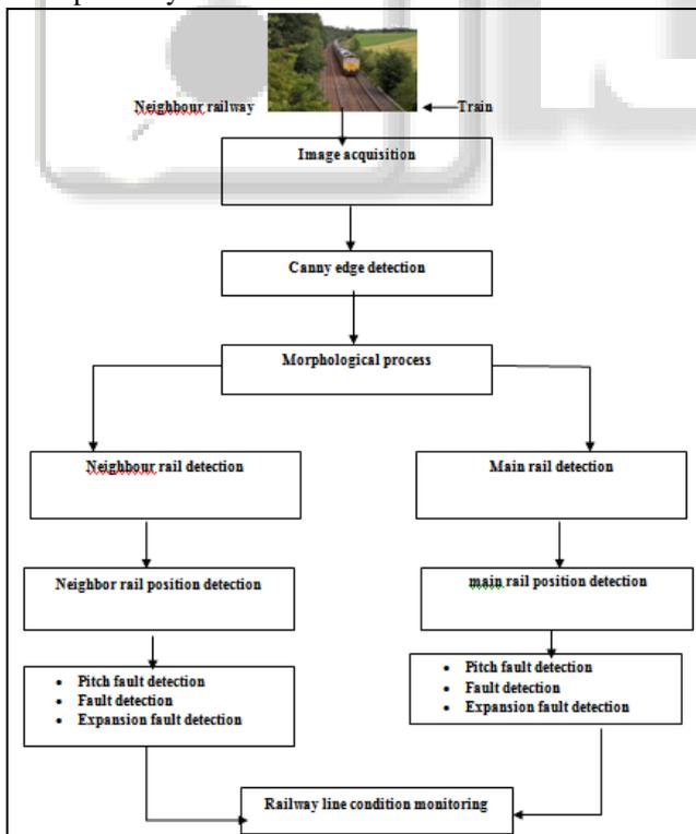
Fig. 2: Block dia. of Rail Defect Detection System
