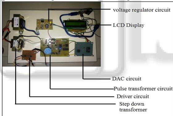
Fig. 5: Hardware Part of controller circuit diagram
