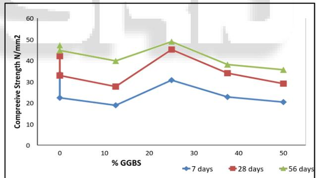
Fig. 3: Compressive Strength of Concrete with 20% Pond Ash
