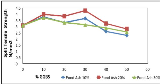
Fig. 5: Split Tensile Strength of Concrete
