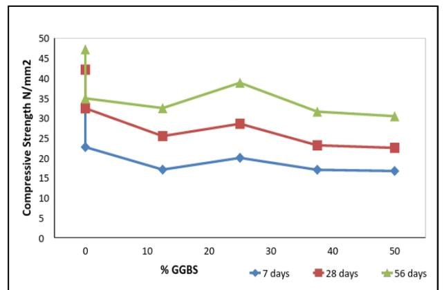
Fig. 4: Compressive Strength of Concrete with 30% Pond Ash
