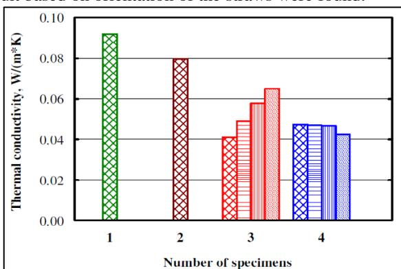
Fig. 6: Measurements of thermal conductivity of straw (1 – specimen made from straw bales; density 100 kg/m<sup>3</sup>; 2 –
