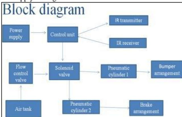
Fig. 11: Block Diagram of Project
