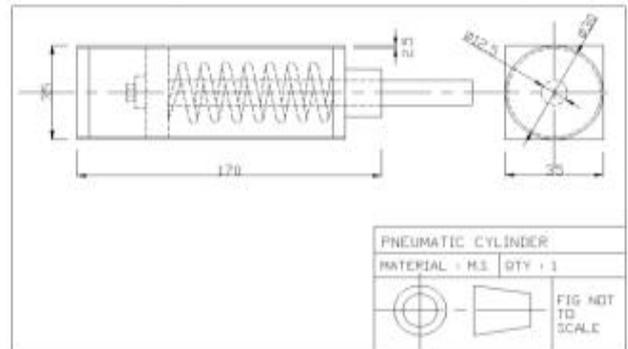
Fig. 5: Pneumatic Cylinder
