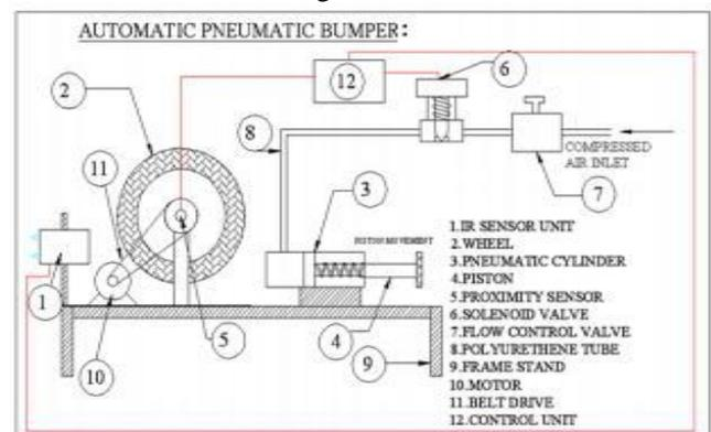
Fig. 13: Automatic Pneumatic Bumper
