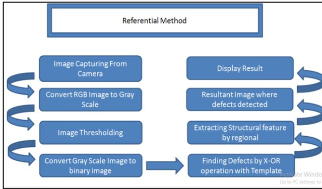
Fig. 1: Steps in PCB Defect Detection
