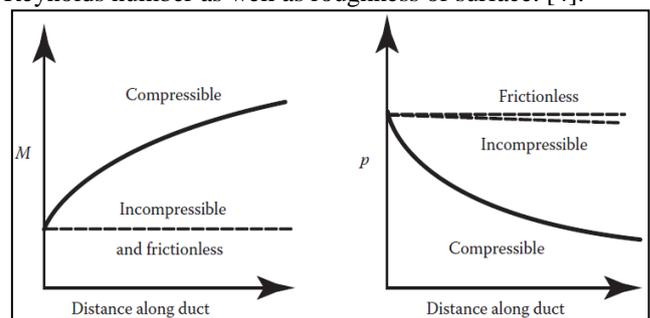
Fig. 1: Effect of Frictional Loss in Mach number (M) and Pressure (p) [5]
