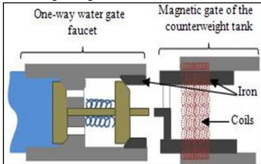
Fig. 3: Water Gate and Magnetic Gate Before Electromagnetic
