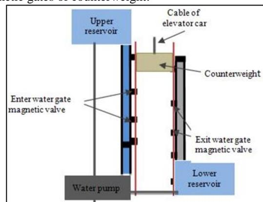
Fig. 2: The Counterweight Operation
