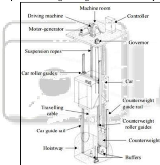
Fig. 1: Main Type of Typical Component of Traction Type Passenger Elevator
