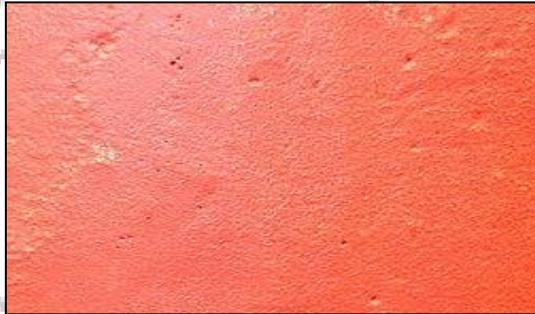
Fig. 5: Blowhole Defect
