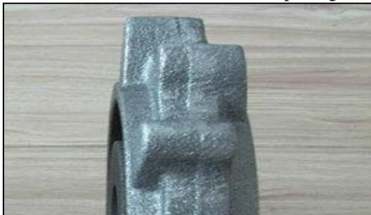
Fig. 6: Mismatch Mold Defect
