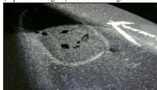
Fig. 3: Shrinkage Cavity Defect
