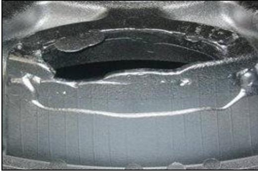
Fig. 4: Misrun Defect
