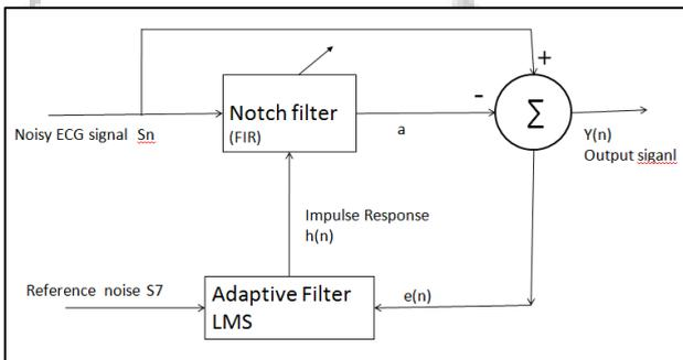
Fig. 2: Block Diagram of Implemented Module without Error Filter
