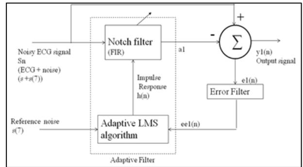
Fig. 3: Block Diagram of Implemented Module with Error Filter
