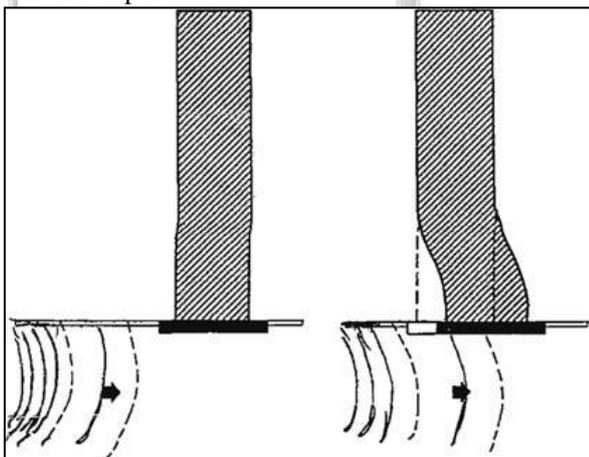
Fig. 2: Showing Action of Seismic Waves on Foundation Soil
