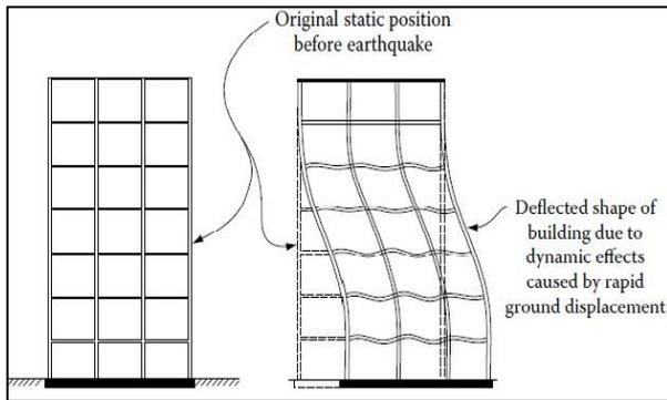
Fig. 1: showing Behavior of Building under Seismic Forces
