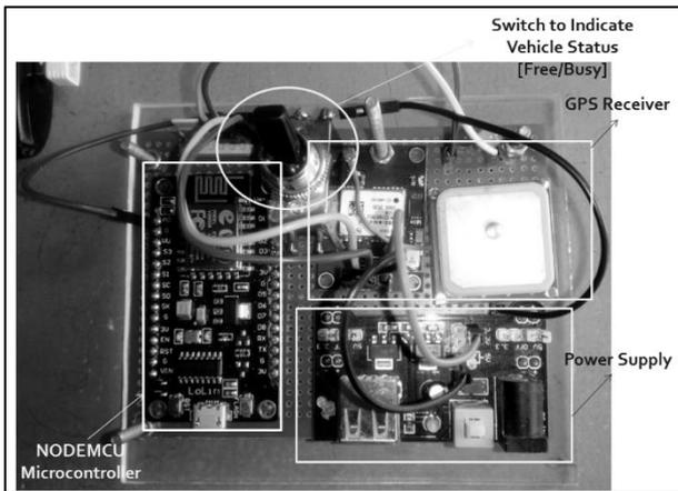
Fig. 3: Working Prototype of VISE
