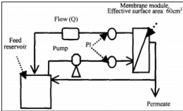
Fig. 2: Schematic Diagram of the Experimental Set-Up of Cross Flow Nano Filtration.
