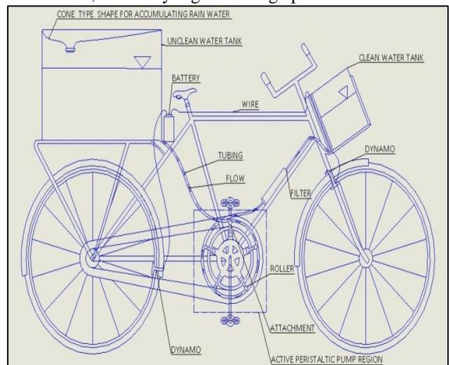
Fig. 1: General Arrangement of the Unit
