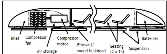
Fig. 3: Hyperloop passenger capsule subsystem notional locations
