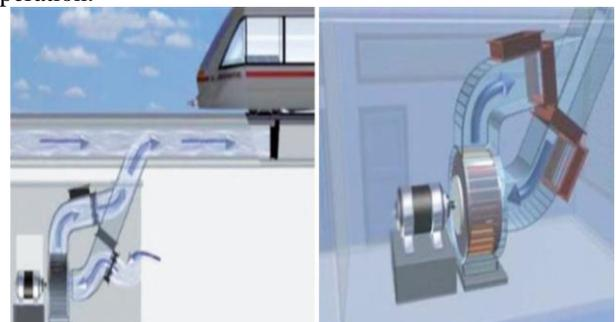
Fig. 1: Propulsion system of Aeromovel
