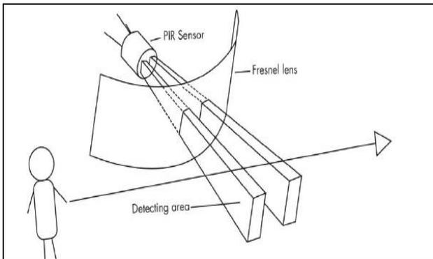
Fig. 1: PIR Motion Sensor
