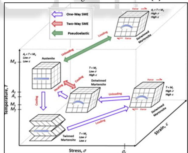
Fig. 2: Shape Memory Phases, Crystals and Effects [2].
