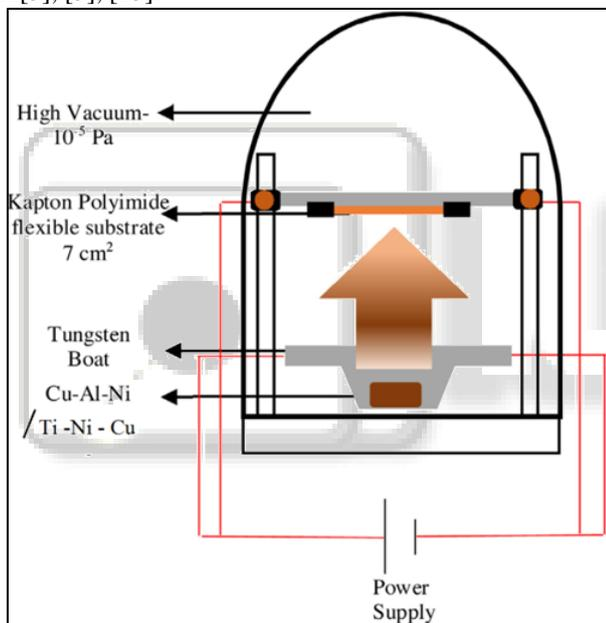
Fig. 3: Thermal Evaporation Setup [3], [5], [13]
