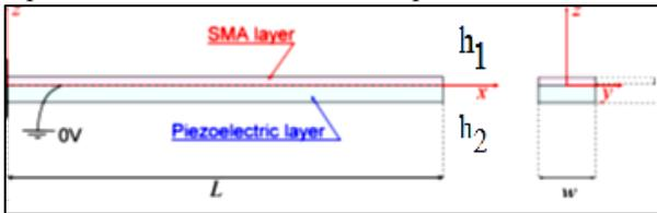
Fig. 5: Schematic View of the SMA-PM Bimorph [20].
