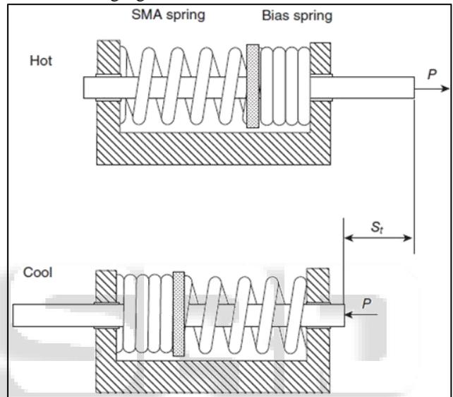
Fig. 7: Show the Proposed Design of SMA Actuator.
