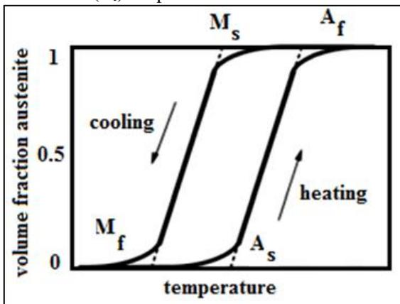
Fig. 1: Generic Graph For A Shape-Memory Material, Showing Transformation Temperatures on Heating and Cooling[7].
