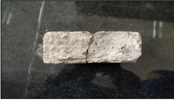
Fig. 1: lab scale model of brick using 40% sludge
