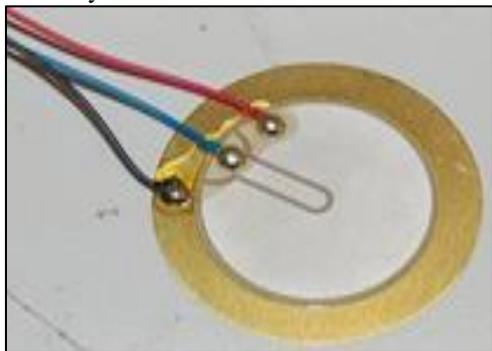
Fig. 4: Piezoelectric Crystal
