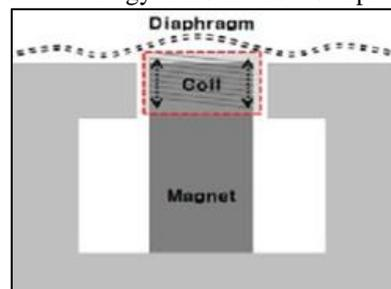
Fig. 2: Noise Energy Generating Device [4]
