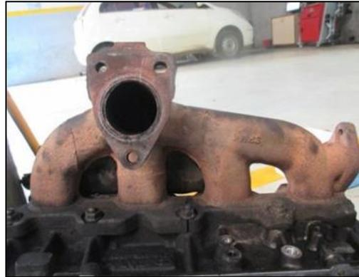
Fig. 1: Exhaust Manifold of Diesel Engine
