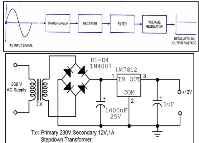
Fig. 7: Regulated Power Supply
