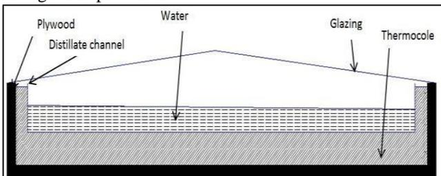
Fig. 1: Single Basin Double Slope Solar Still
