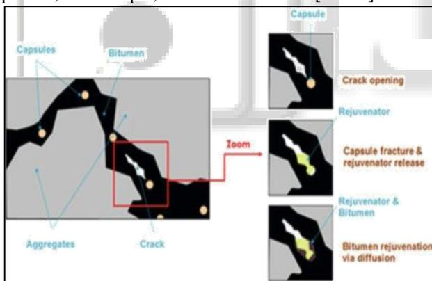
Fig. 1: Self healing by Rejuvenator mechanism
