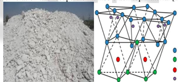
Fig. 2: Nanoclay and its chemical structure
