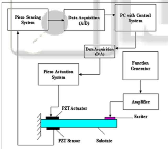
Fig: 1: Block Diagram Of Vibration Control
