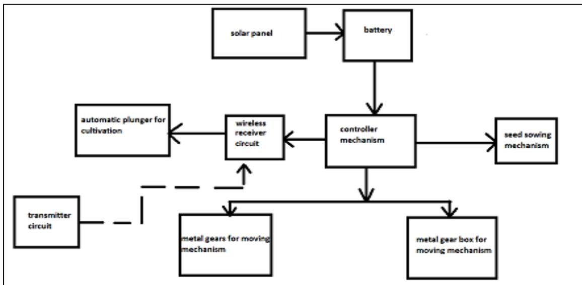
Fig. 1: Block diagram of remote operated farm equipment
