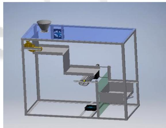
Fig. 2: VTD [Vibro Thermal Disinfestor]
