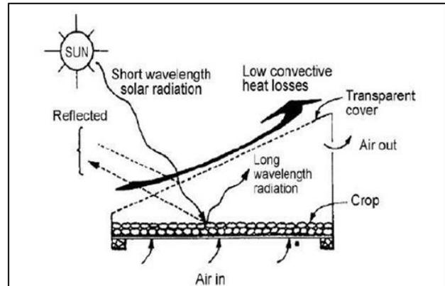
Fig. 1: direct type solar dryer direct type solar dryer, It is found that time required for drying [3]
