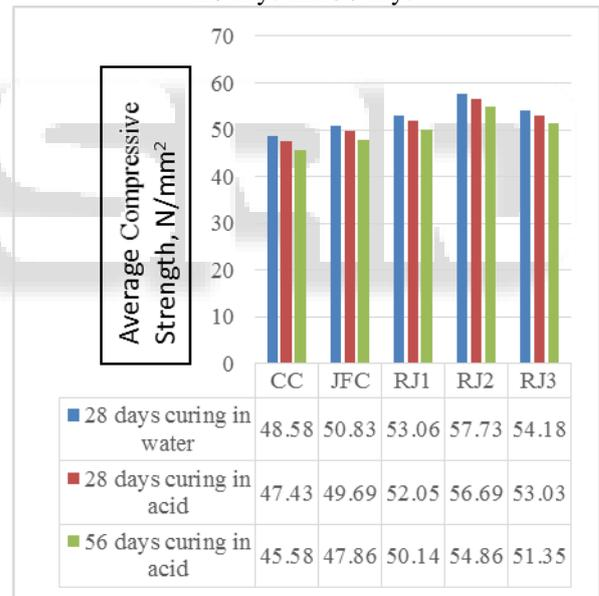
Fig. 5: Average compressive strength of the specimen under acid test after 28 days and 56 days
