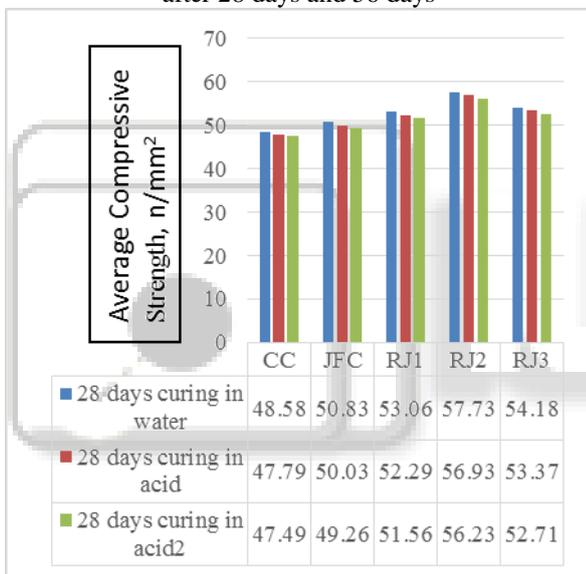
Fig. 7: Average compressive strength of the specimen under chloride test after 28 days and 56 days
