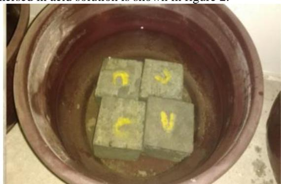
Fig. 2: Concrete specimen immersed in acid solution
