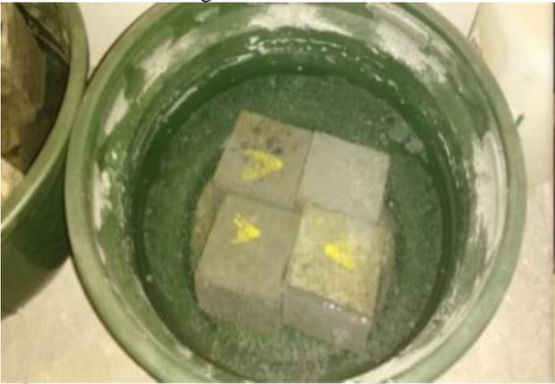
Fig. 3: Concrete specimen immersed in chloride solution
