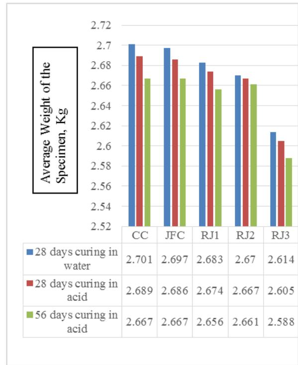
Fig. 4: Average weight of the specimen under acid test after 28 days and 56 days
