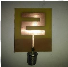
Fig. 8: z shape fabricated MPA(Front)
