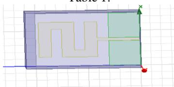
Fig. 1: Z shape antenna
