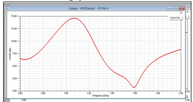
Fig. 5 :Frequency Vs VSWR of Z shape antenna (Graph)
