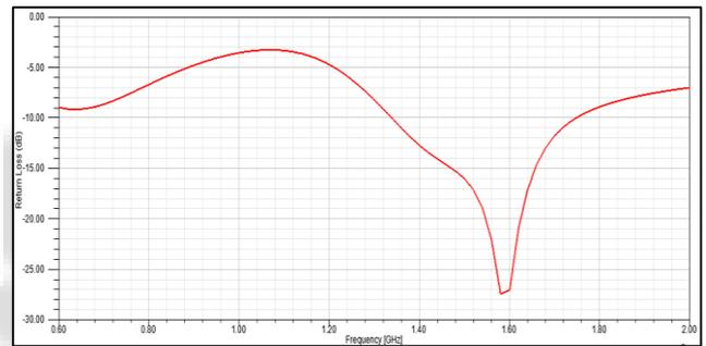
Fig. 4: Return loss of Z shape Antenna (graph)
