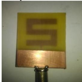
Fig. 9: fabricated MPA (Back)
