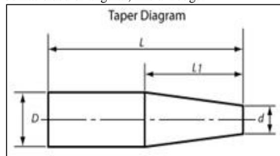
Fig. 1: A taper is a uniform change in a cylinder's diameter when measured along its axis. The section labelled  $L_1$  shows a taper.
