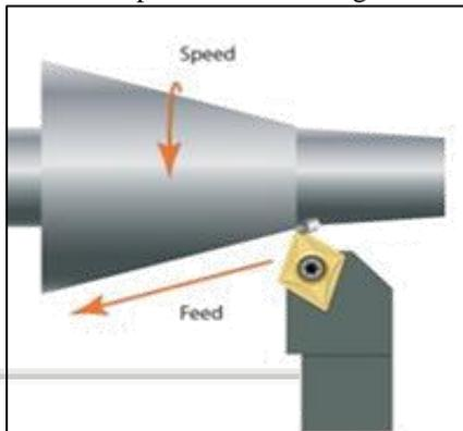
Fig. 3: A taper is turned on a lathe by cutting at an angle relative to the workpiece centerline.
