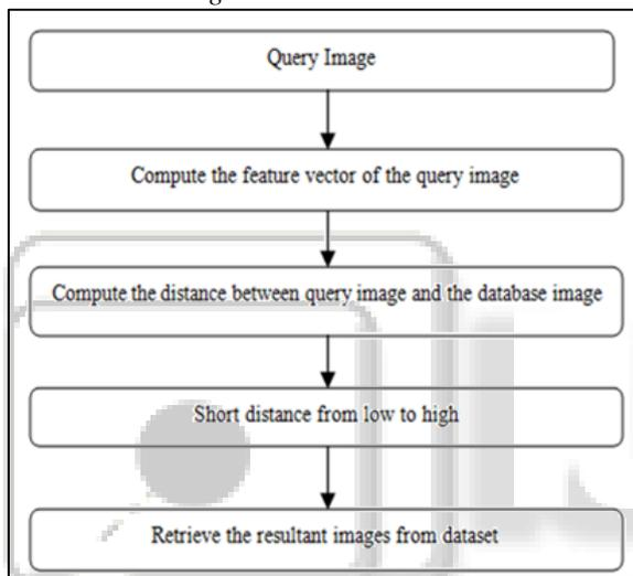
Fig. 3: Flowchart for feature matching process
