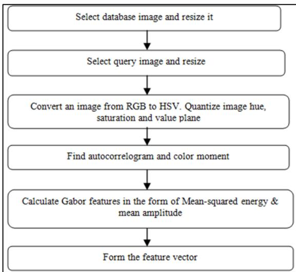
Fig. 3: Flowchart for feature extraction process
