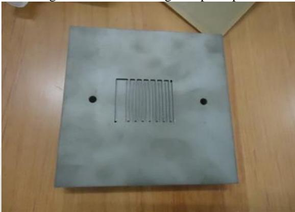
Fig. 2: Graphite bipolar plate
