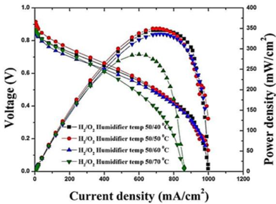
Fig. 6: Graph 2 Humidification temperature variation-cathodes
