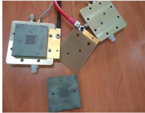
Fig. 4: single cell PEMFC assembly
