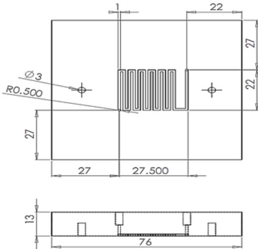
Fig. 1: Detailed drawing of bipolar plate
