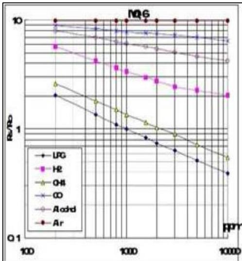
Fig. 3: Sensitivity Characteristics of MQ-6 Gas Sensor
