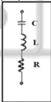
Fig. 2: Single tuned passive filter
