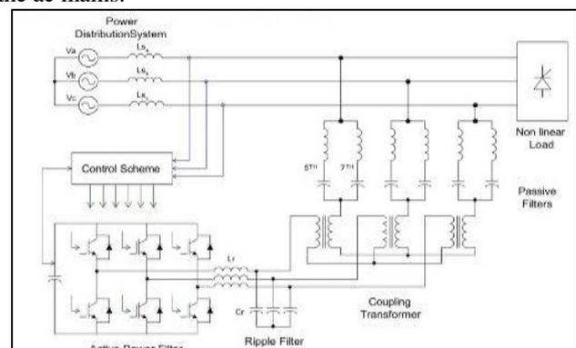
Fig. 1: Circuit diagram of the HAPF
