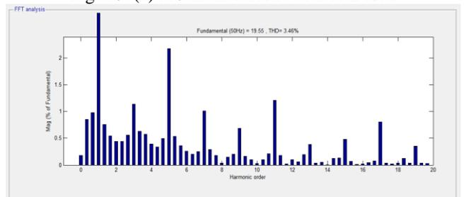
Fig. 11: (b) AC mains voltage response with %THD
