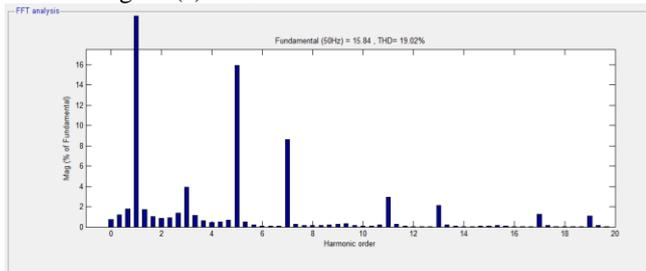
Fig. 6: (b) AC mains voltage response with %THD
