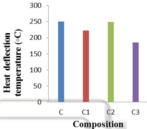
Fig. 3: comparison composites on the basis of HDT
