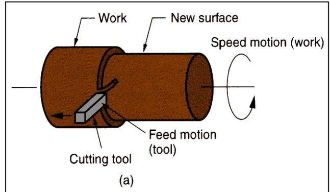
Fig. 2: Cutting Process in Turning
