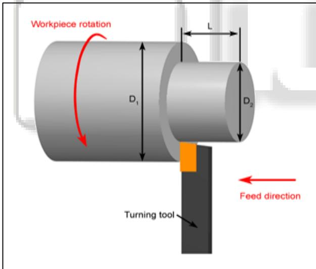
Fig. 1: Turning Process
