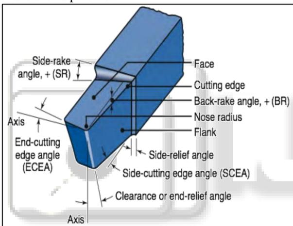
Fig. 3: Tool Geometry
