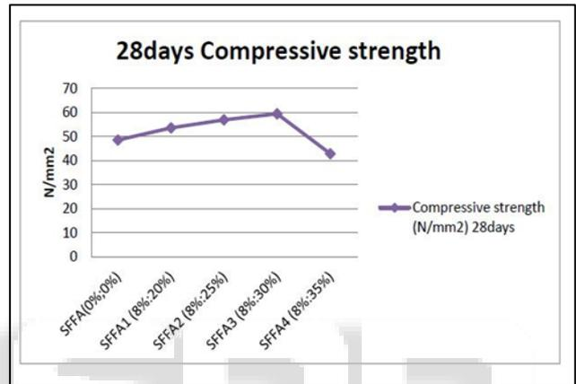
Fig. 4: Compressive strength in 28 days of FA and Silica fume HSC mixes
