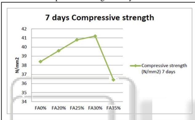
Fig. 1: Compressive strength in 7 days of Fly Ash HSC mixes
