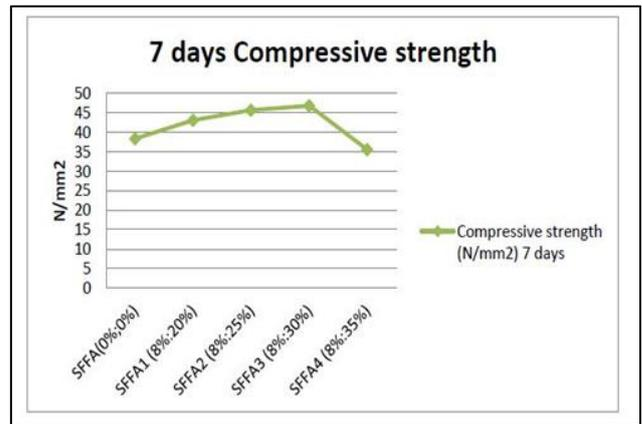
Fig. 3: Compressive strength in 7 days of FA and SF HSC mixes
