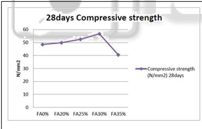
Fig. 2: Compressive strength in 28 days of Fly Ash HSC mixes
