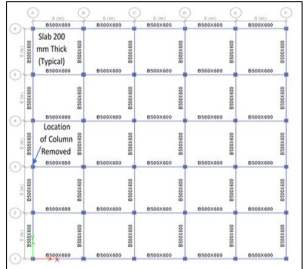
Fig. 4: Reinforced Concert Building Plan and Location of Column Removed
