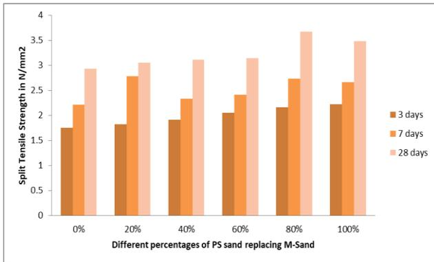
Fig. 4.2: Shows the variation of Split Tensile Strength at 3, 7 and 28 days for M20 grade concrete with different percentages of PS sand replacing M-Sand.
