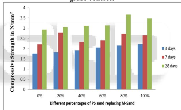
Fig. 4.1: Shows the variation of Compressive Strength at 3, 7 and 28 days for M20 grade concrete with different percentages of PS sand replacing M-Sand.
