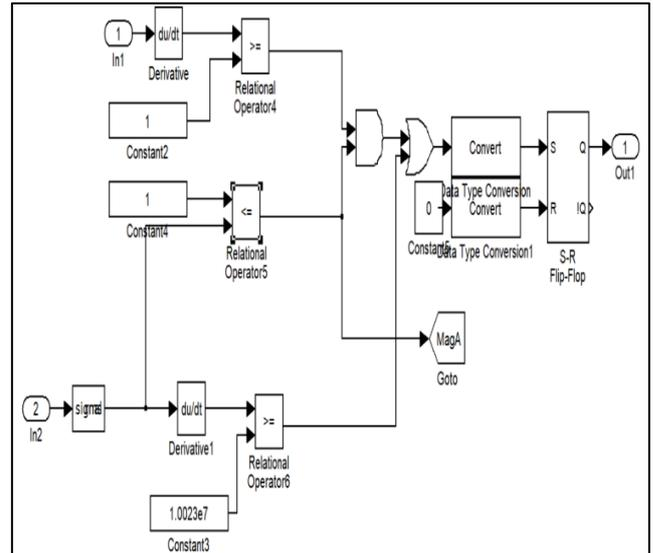
Fig. 5: Fault Detection Module
