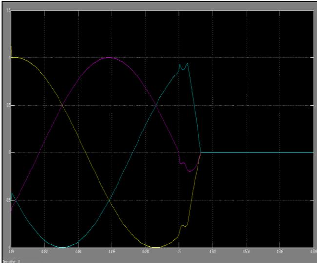
Fig. 3(c): Inverter fault current with proposed fault controller
