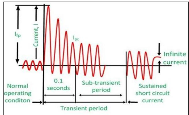
Fig. 1: Transient Behavior of Short Circuit Current
