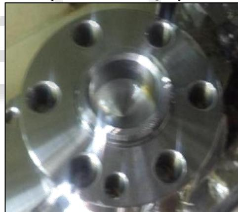
Fig. 3: The Picture of Part of Crankshaft after Implementation of MQL System
