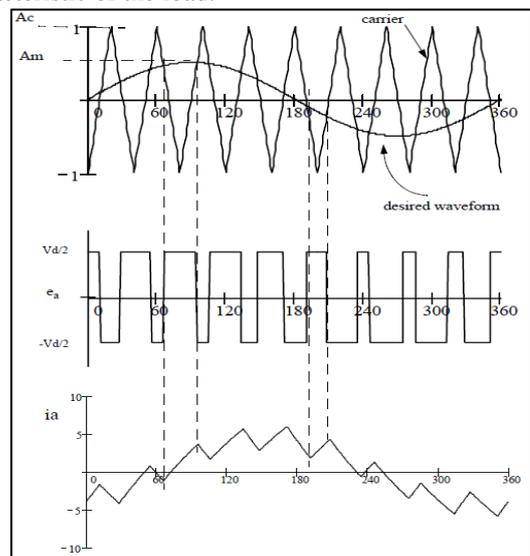
Fig. 8: Principle of Pulse Width Modulation
