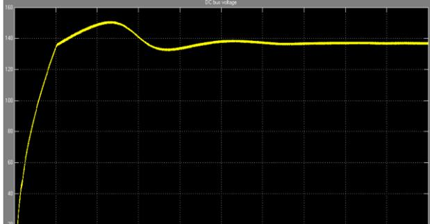
Fig. 13: Output from CUK Converter
