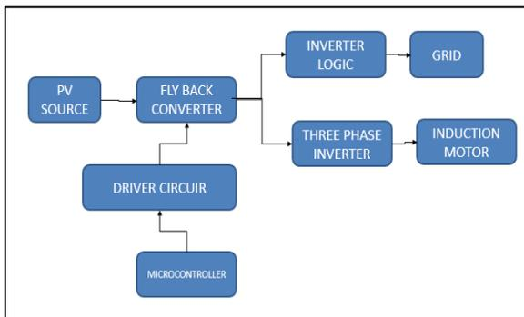
Fig. 4: Block Diagram of Existing System
