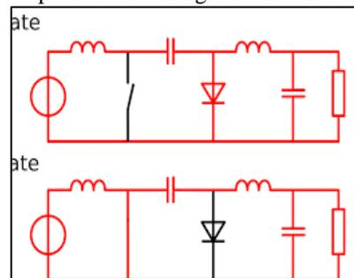
Fig. 3: CUK Converter Operation
