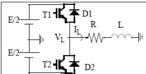
Fig. 7: Simple Voltage Source Inverter
