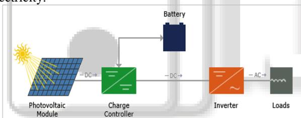
Fig. 6: PV System Powering AC Loads With Battery
