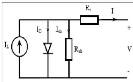
Fig. 1: Standard Equivalent Circuit of PV
