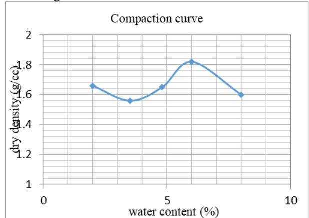
Fig. 4.4: Compaction Curve for Sand
