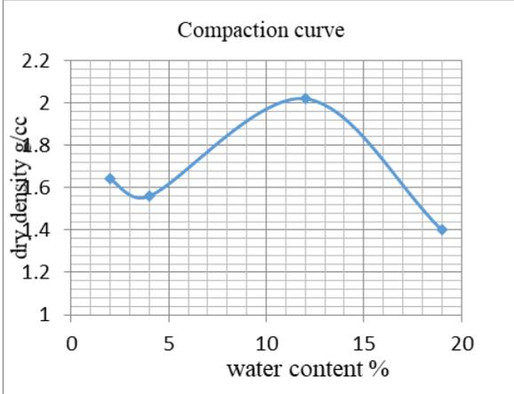
Fig. 4.2: Compaction Curve of Crusher Dust
