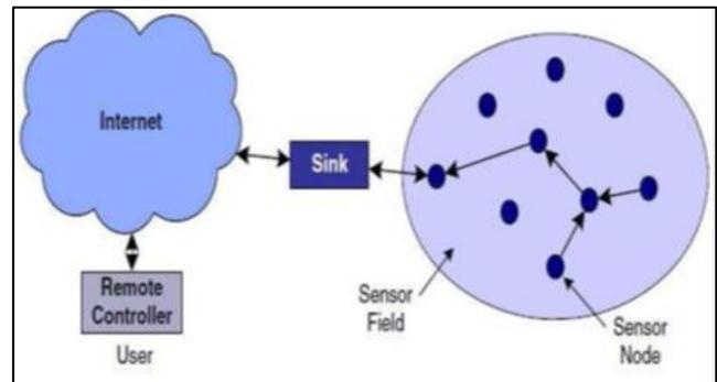
Fig. 1: Architecture of a sensor Node<sup>[6]</sup>
