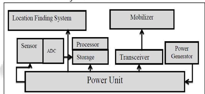
Fig. 2: Components of a sensor node<sup>[7]</sup>
