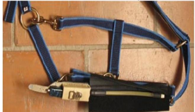
Fig. 2: Noseband halter which is used for recording.
