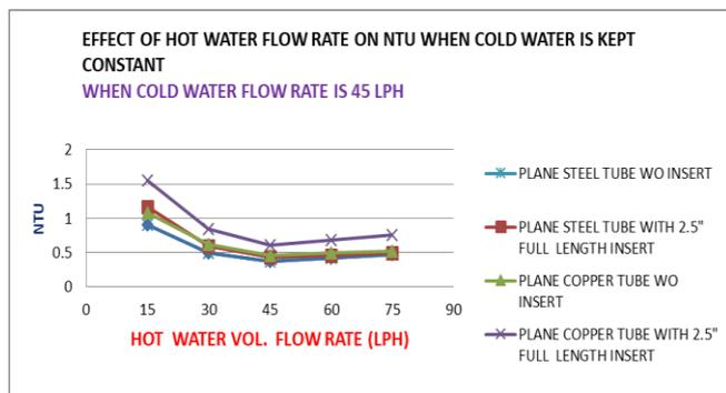
Graph 1: Comparative Analysis Of NTU When Cold Water Is Constant At 45 LPH For Plane Steel Tube & Plane Copper Tube DPHE Without Insert And With 2.5” Full Length Insert In Counter Flow Arrangement.
