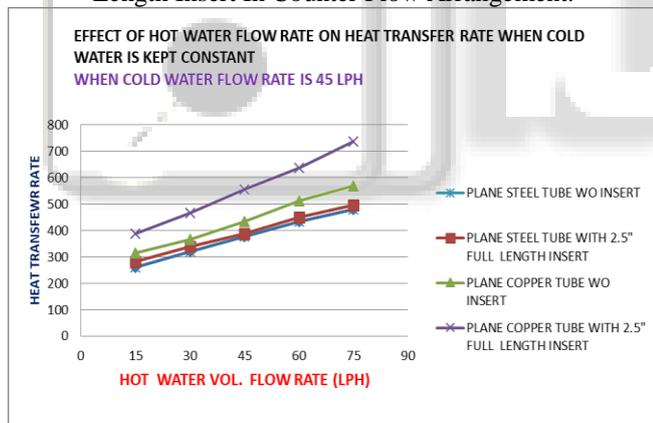
Graph: 2 Comparative Analysis Of Heat Transfer Rate In Cold Fluid When Cold Water Is Constant At 45 LPH For Plane Steel Tube & Plane Copper Tube DPHE Without Insert And With 2.5” Full Length Insert In Parallel Flow Arrangement.
