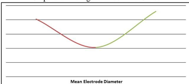
Graph 3: Breaking Load v/s Mean Electrode Diameter
