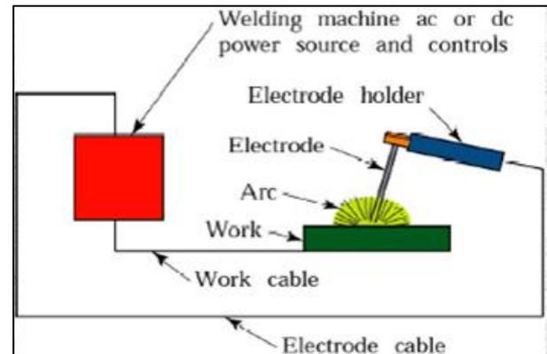
Fig. 2: Experimental setup of electric arc welding
