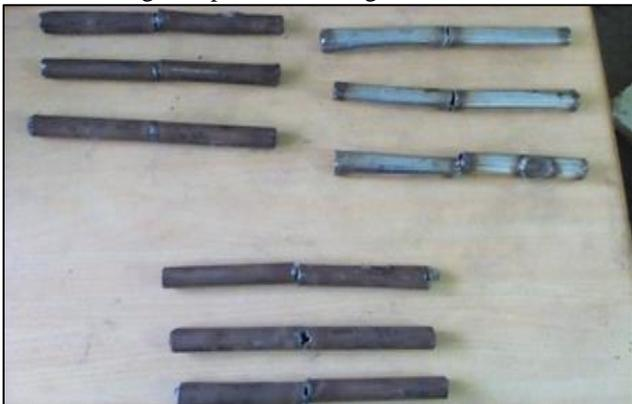
Fig. 4: Specimen after Tensile Test
