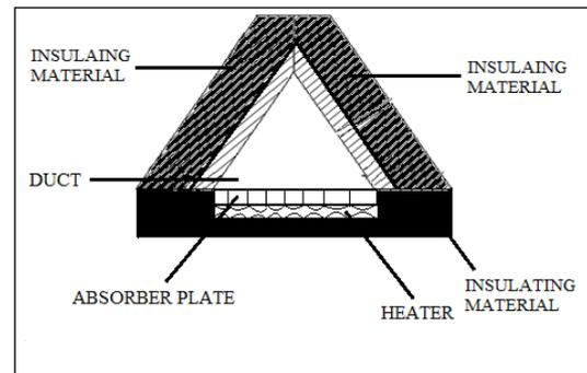
Fig. 2.1: Sectional View of the Duct
