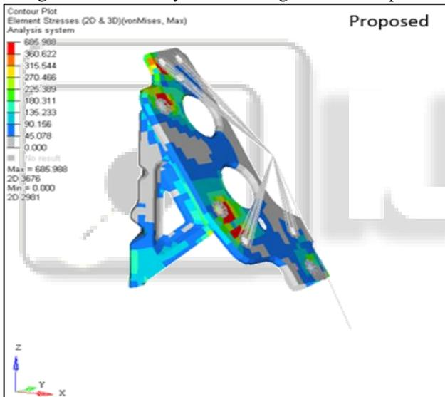
Fig. 1.5: Stress analysis of existing proposed pedal
