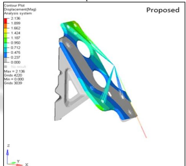
Fig. 1.7: Displacement analysis of existing Accelerated pedal
