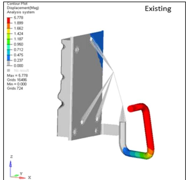
Fig. 1.6: Displacement analysis of existing Accelerated pedal
