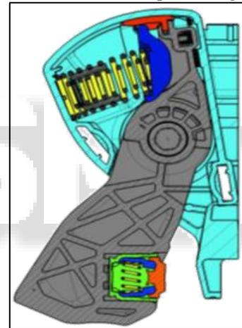
Fig. 1.2: Cross-section of accelerated pedal System
