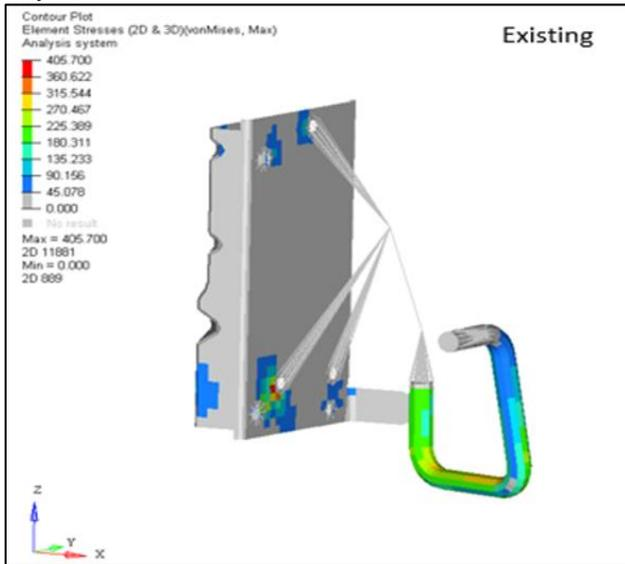
Fig. 1.4: Stress analysis of existing Accelerated pedal
