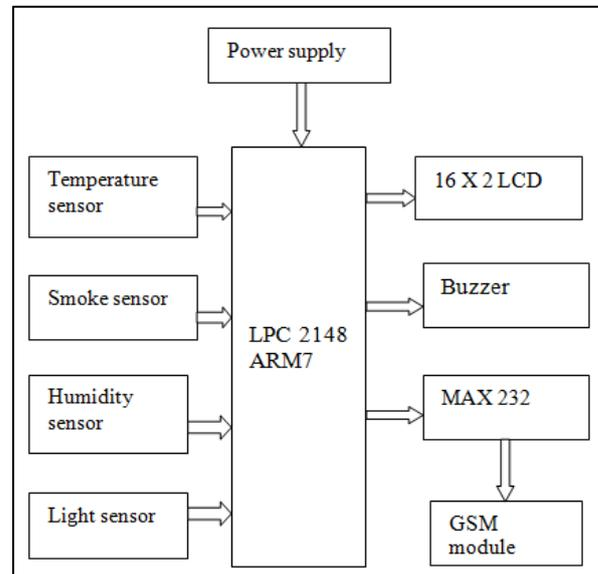
A GSM modem duly interfaced to the MC through the level shifter IC Max232. The SIM card hooked up GSM modem upon receiving digit command through SMS from any cellular smartphone ship that statistics to the MC thru serial verbal exchange. While this system is accomplished, the GSM modem gets command 'STOP' to broaden an output on the MC, the contact factor of which are used to disable the ignition switch
