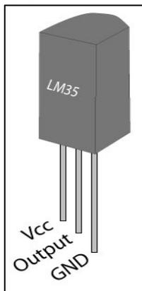
LM35 is a precision IC temperature sensor with its output proportional to the temperature (in oC). The sensor
